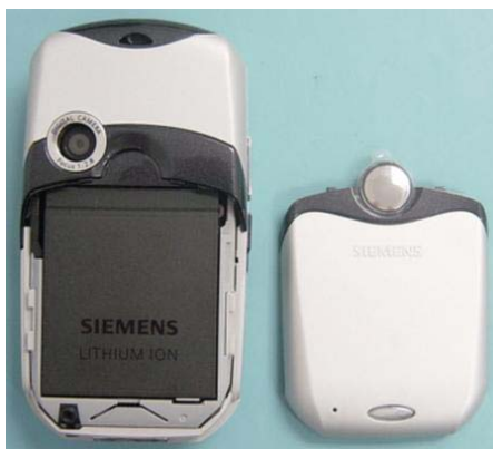
Remove Battery cover.
