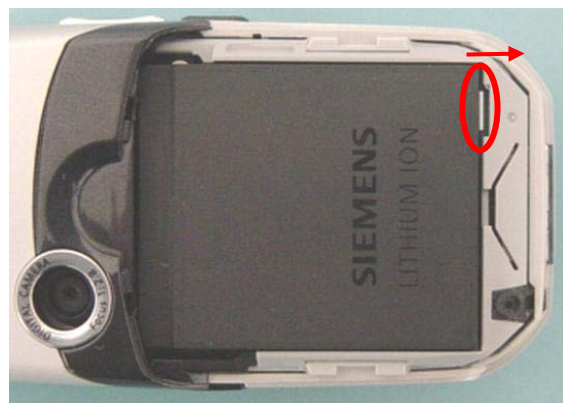
Remove Battery – push the catch in the direction shown.
