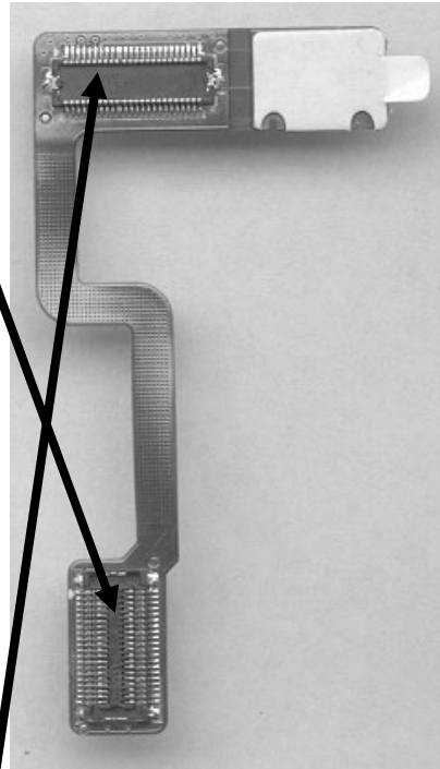
LCD FPCB 40 pin and 48 pin Connector
