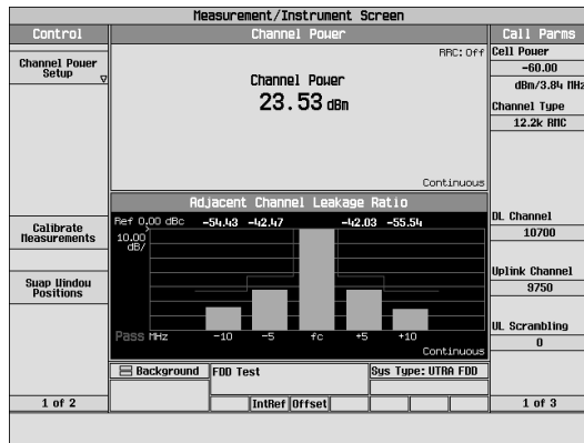
Fig. 4-34-1 Output Level at RF test connector ( W100)
