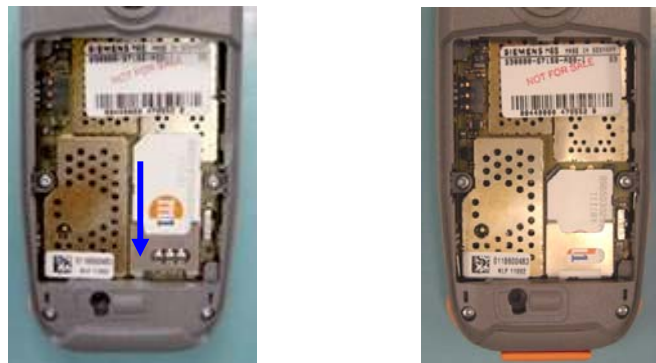
Installation of the SIM card
