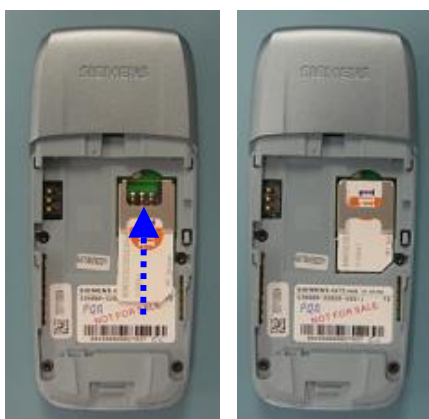
Installation of the SIM card
