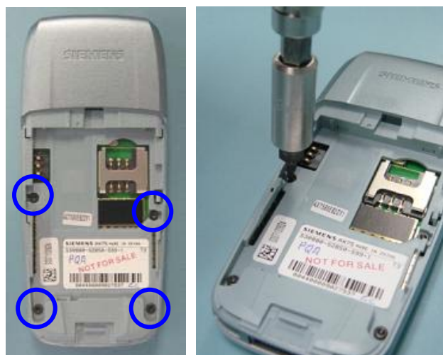
Remove the 4 screws (as indicated) with T5 Plus screw driver.
