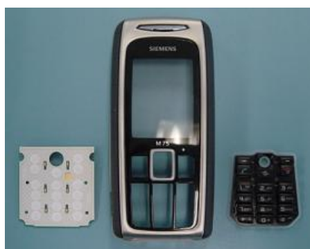
Remove MMI and Keypad
