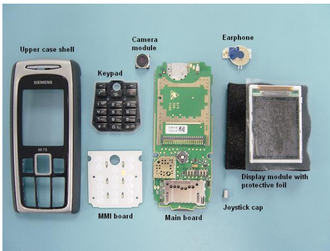
Fully disassembled M75 - upper parts (top) and lower parts (bottom).
