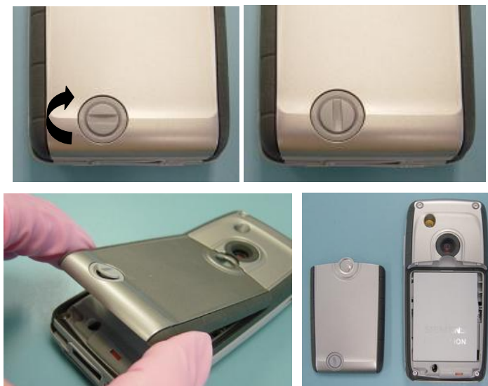
Remove Battery cover
