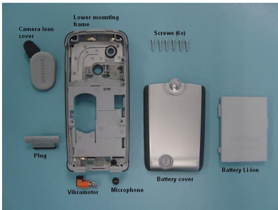
Fully disassembled M75 - upper parts (top) and lower parts (bottom).
