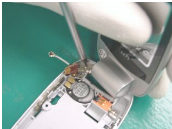
Tighten 1 screw on shaft (T3, 7cNm)
