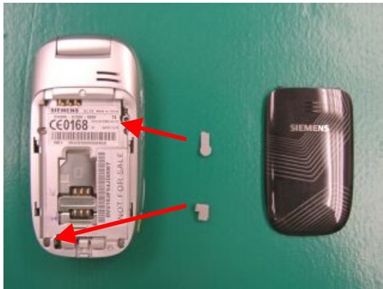
Open battery cover and remove test and antenna pad.
