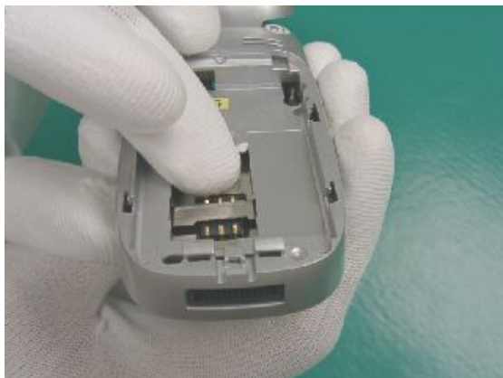
Push the main PCB from SIM connector and carefully lift.
