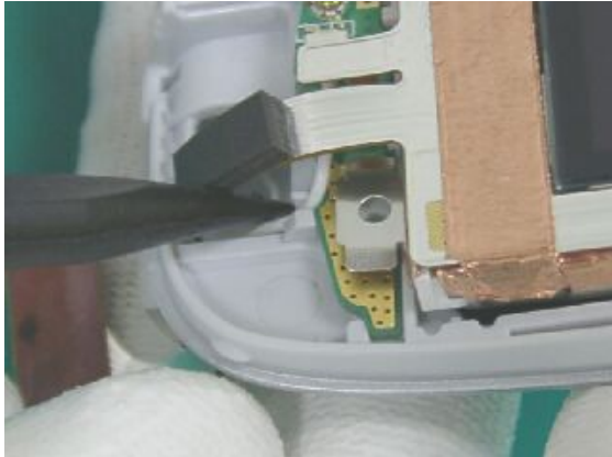
Adjust antenna cable in front of LCD cable
