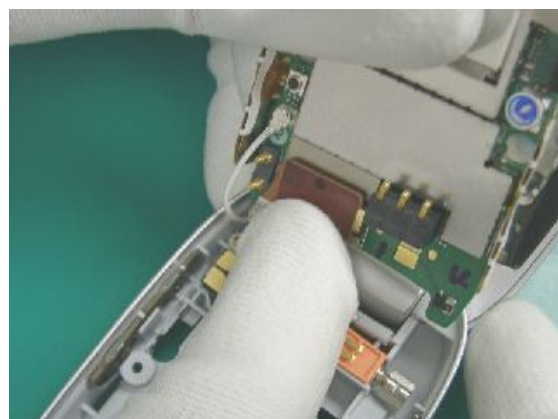
Plug in flex cable and arrange antenna cable to fix along the side of speaker spring
