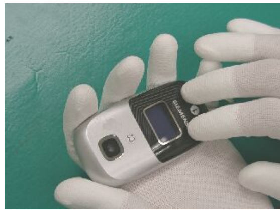
Slight click LCD top case and remove LCD top case
