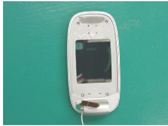
Unscrew 4 screws on LCD base case
