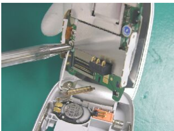
Lock antenna cable to PCB
