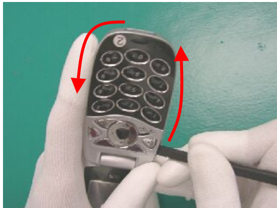
Insert the opening jig into the key set and slide along the sides.
