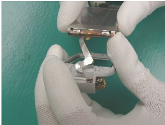
Swirl LCD cable and pull out through the hole
