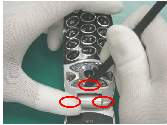
Carefully separate 3 hooks of the key set.
