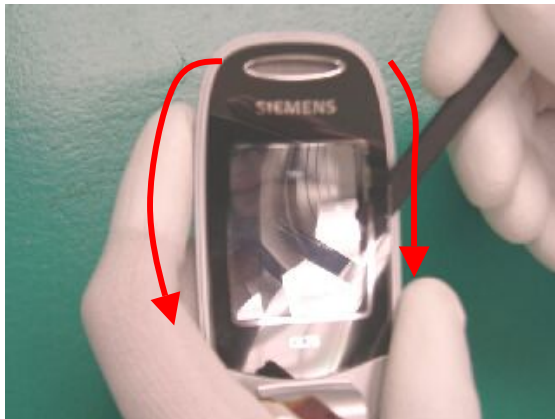
Insert the Jig between LCD base case and LCD lens and slide around to remove LCD lens
