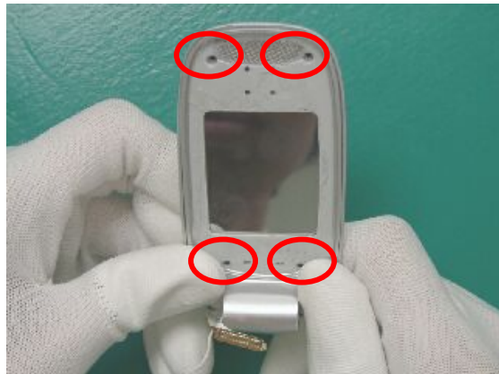
Press along the sides and tighten 4 screws on LCD base case (T3, 7cNm)
