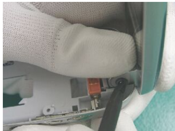
Align left side of LCD case, insert LCD hinge on right side and press to fix LCD case into base case
