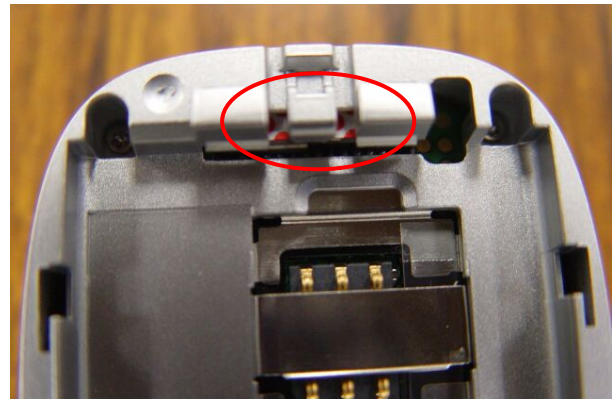
Water indicator ( can be seen through the base case )
