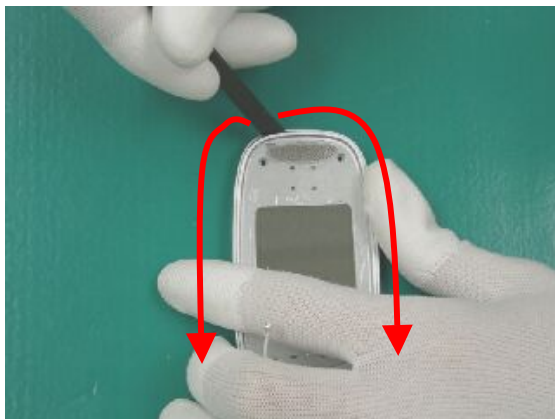
Insert the jig into the gap and slide around to dismount LCD base case
