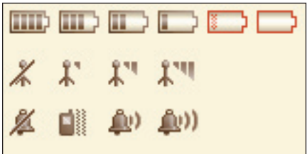
2. Sample icons for ringer, battery and Signal Strength, showing states equivalent to: 'none, low, medium, full'
