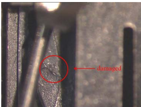
Lock mechanism damaged
