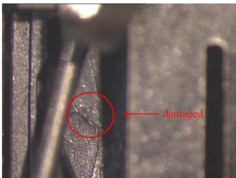
Lock mechanism damaged
