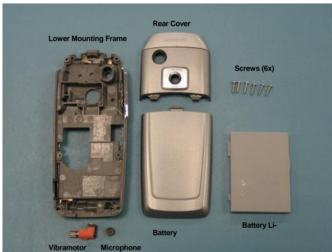
Fully disassembled CX75 - upper parts (top) and lower parts (bottom).
