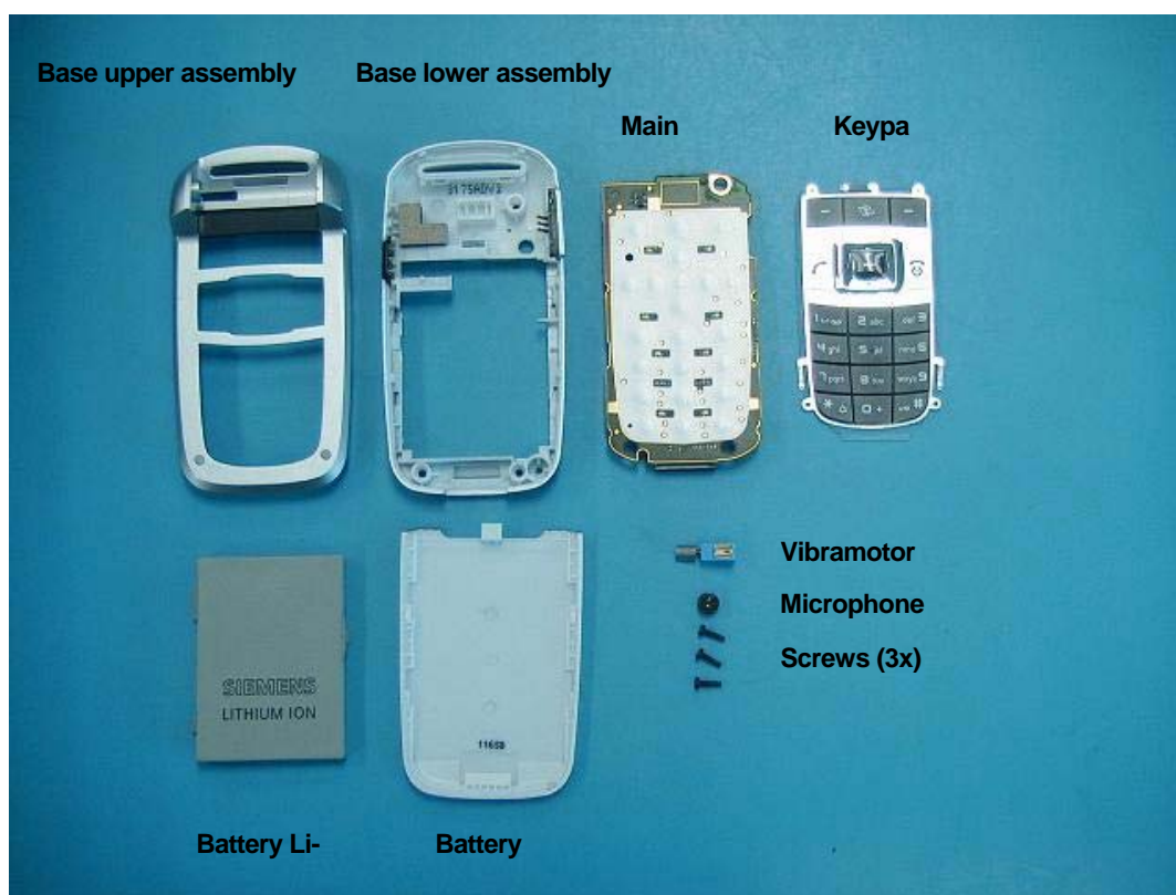
Fully disassembled CF75 - Lower parts
