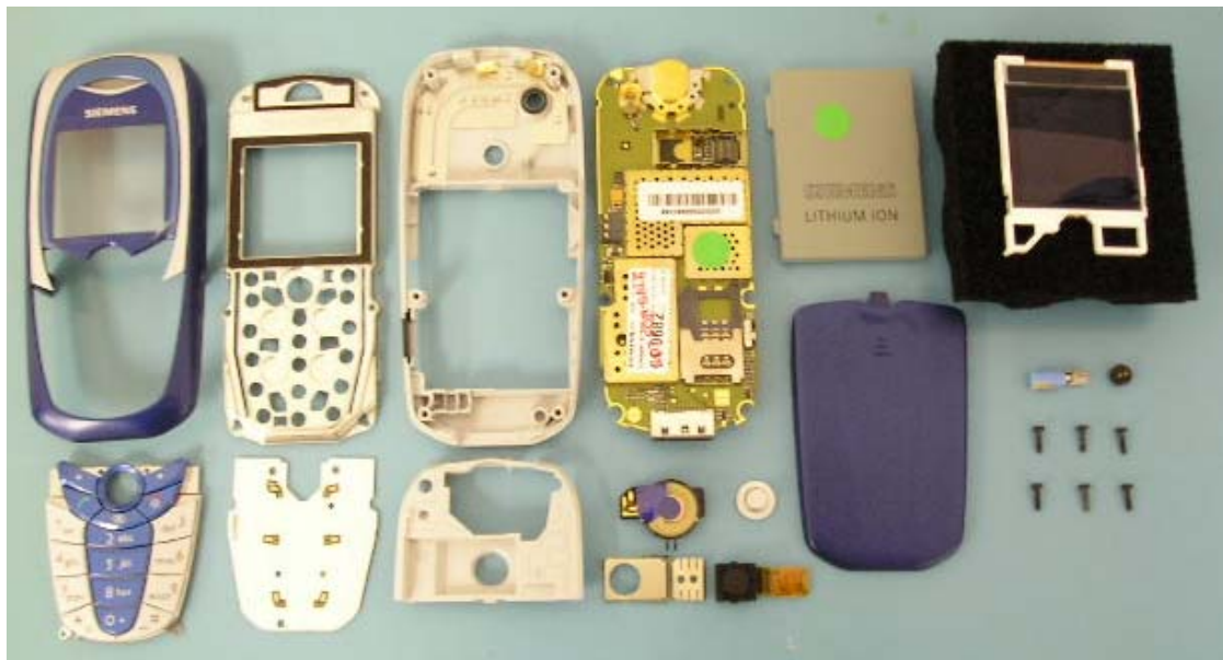
Fully disassembled C65
