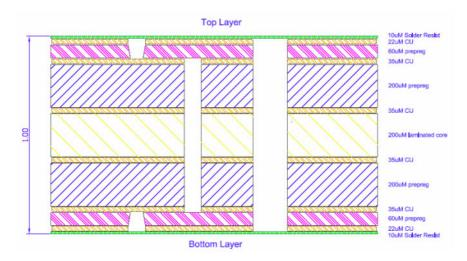
Surface Finishing: Chemical Gold Plate Ni 5 uM / Au 0.1 uM
