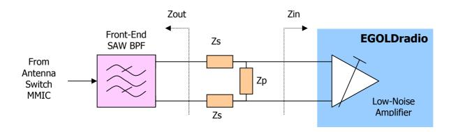
RF matching components might be either calculate by analytical/simulation approach or by trial-and-error.
