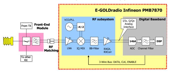
For each of the 4-band (GSM900, DCS1800, PCS1900 and GSM850), the RX path is mainly composed by similar functional blocks, namely:
