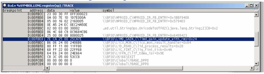
■ Sometimes, expecially when traps occur or when the system stops in the Apoxi area, a 2 byte offset has to be applied to the SP in order to see the correct stack:
