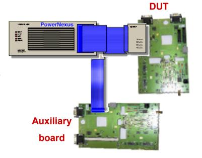
This approach is useful to trace DUT in power saving mode, because it prevents the JTAG connector from keeping the MS awaken and lengthens the temporal duration of the backtrace (which is otherwise ca 2 seconds).
