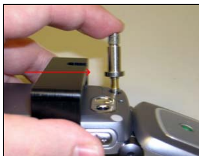
Fig.1 Slide the holder against the RF adapter.
